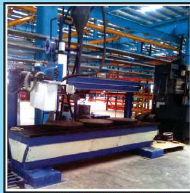
3 STATION SERVO BASED SAW WELD OVERLAY SYSTEM
