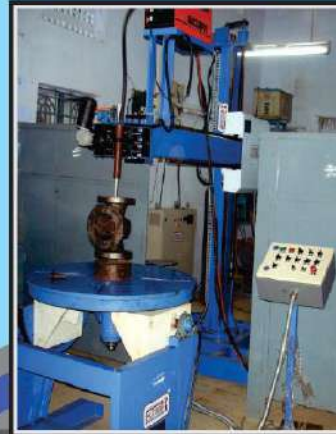
GATE VALVE WELDING SYSTEM
