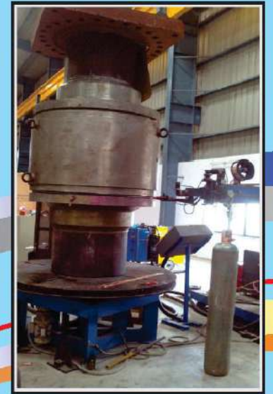
BALL VALVE ROOT TIG WELDING SYSTEM
