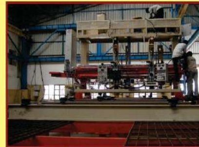
PANEL WELDING SYSTEM FOR BOILER MANUFACTURING
