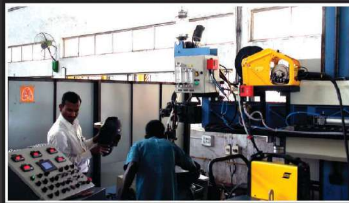
PTA CUM MIG WELD OVERLAY SYSTEM FOR VALVE COMPONENTS
