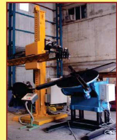
COLUMN & BOOM MANIPULATOR FOR SS BELLOWS WELDING
