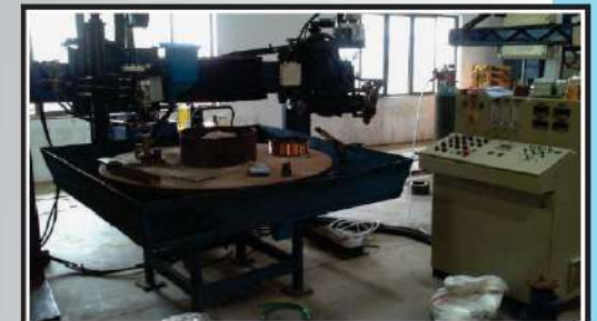
PTA CUM SAW WELD OVERLAY SYSTEM FOR VALVE COMPONENTS
