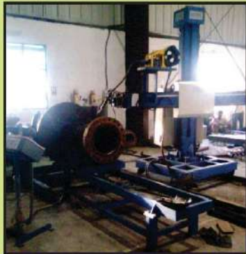
PTA CUM MIG WELD OVERLAY SYSTEM FOR VALVE COMPONENTS
