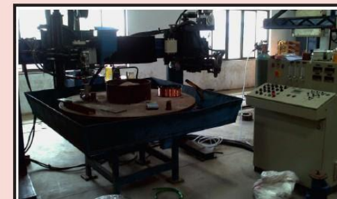
PTA CUM SAW WELD OVERLAY SYSTEM FOR VALVE COMPONENTS
