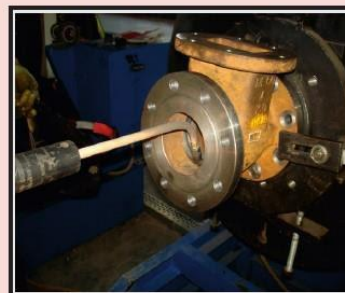
MECHANIZED SEAT RING SEAL WELDING SYSTEM
