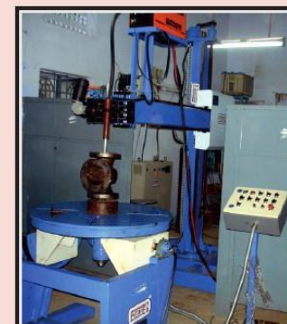
GATE VALVE WELDING SYSTEM
